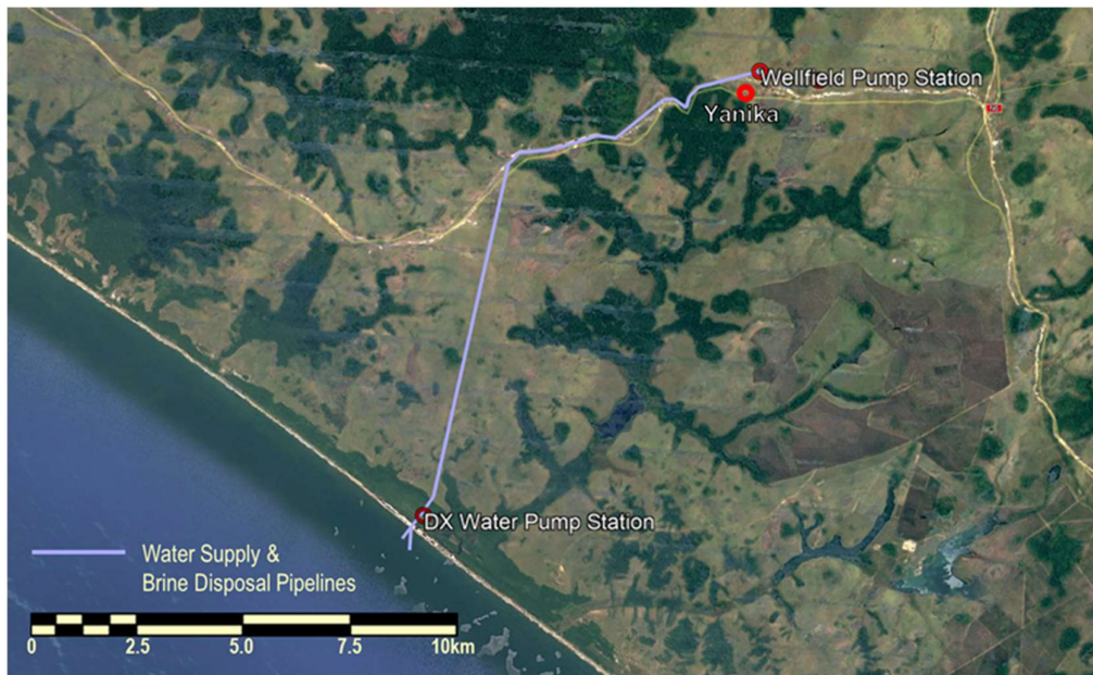
Figure 14 : Proposed route for brine discharge and sea water supply pipelines
