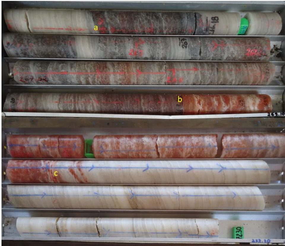
Figure 16. Photograph of (PQ size) core from an intersection of Upper Seam in drill-hole EK_38. The seam is partially replaced; the upper part of the seam (a to b) is Sylvinitic (USS) and the lower part (between b and c) is Carnallitic (USC). Classified as 'type B' seam (as per Table 4 below). The easily identifiable and abrupt nature of the contacts is visible.
