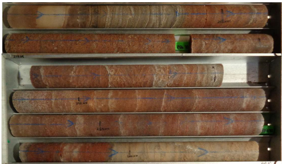
Figure 1 - Whole PQ-sized core shortly after drilling, Sylvinite clearly visible as the orange-red rock type. The seam in this example is the Hangingwall Seam Sylvinite comprised between 50 and 60% sylvite . The easily identifiable and abrupt nature of the contacts is visible.
